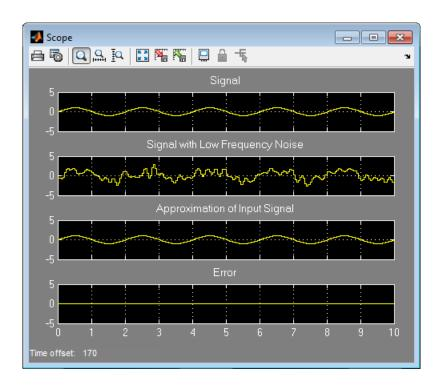
You have now created a model capable of adaptive noise cancellation. So far, you have learned how to design a lowpass filter using the Digital Filter Design block. You also learned how to create an adaptive filter using the LMS Filter block. The DSP System Toolbox product has other blocks capable of designing and implementing digital and adaptive filters. For more information on the filtering capabilities of this product, see "Filter Design" and "Filter Analysis".
