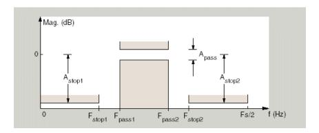
In this example, a sampling frequency of Fs = 48 kHz is used. This bandpass filter has the following specifications, specified here using MATLAB code:
